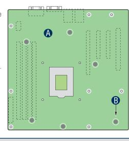
A. Open the Socket Lever B. Open the Load Plate
