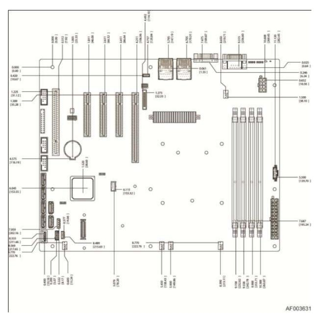
Figure 6. Intel<sup>®</sup> Server Board S1200BTL/S1200BTLRM – Major Connector Pin Location (1 of 2)
