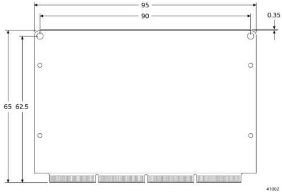
Figure 11. Integrated Heat Shield Side
