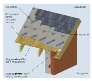
Figure 8b Verges – Fully Supported Horizontal Installation with Natural Slates
