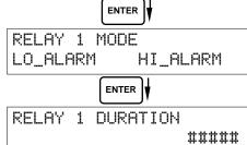
Select the desired Relay Activation. Low: Relay activates when reading is below setpoint.
