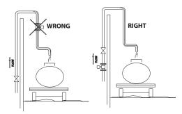
Do not install in a vertical, downward position. Position "On/Off" valves on downstream side. *Figure 13: Position valves on downstream side*
