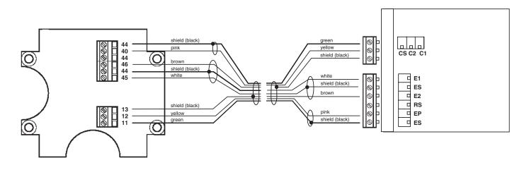
Figure 17: Wiring for remote configuration
