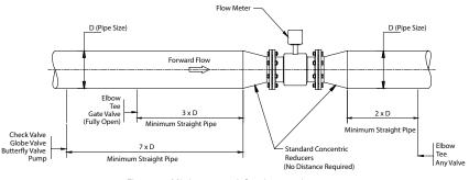
Figure 8: Minimum straight pipe requirements
