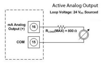
Figure 19: Analog output wiring diagram
