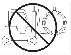
Do not lift detector with forklift.
