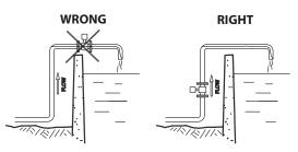
Figure 12: Incorrect meter placement
