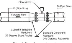
Figure 9: Pipe reducer requirements
