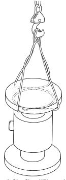
Figure 3: Sling-Rigged lifting methods
