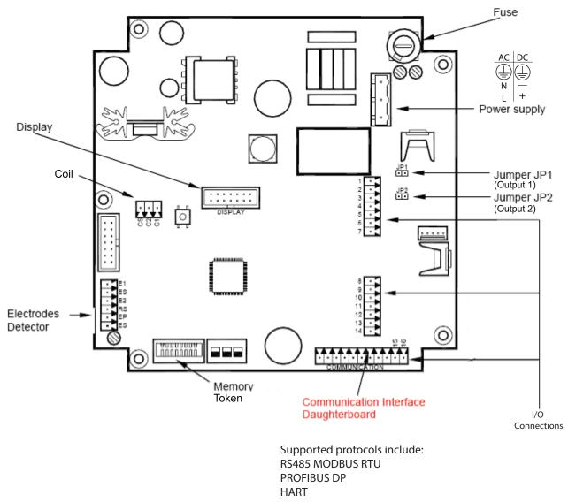
Figure 18: Configuring input/output
