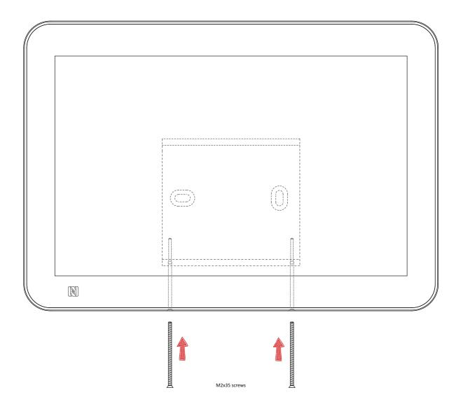
A When installed on the NAPOE109kt or NAPOE109ft products having a mounting bracket with a POGO connector, before mounting the screws to lock the device, check that the TAB10b device is installed on the NAPOE109kt or NAPOE109ft products stricly on the vertical position else some unexpected power supply issue could be faced.
