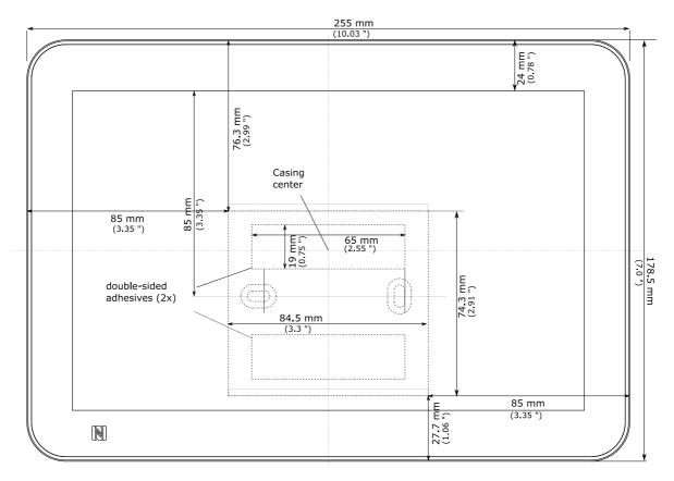
▲ Clean carefully the surface before sticking the adhesive tapes.
