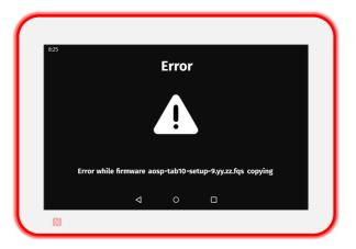
One of these messages could occur when the .fqs firmware is corrupted or when the USB storage device has been removed when the copy was still in progress. If required, download again the .fqs firmware from the Qeedji Website and try again. If the problem persists, contact support@qeedji.tech.
