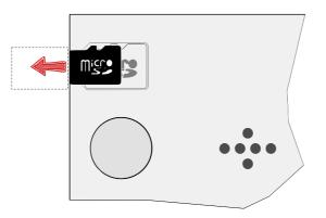
It may be required to lift the micro SD card so that it can enter into the connector. Press a little on it to tilt it.
