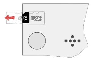
Step 3: When the spring of the SD card connector is responding properly, helped with a pen, push the micro SD card towards the connector until hearing a clic.
