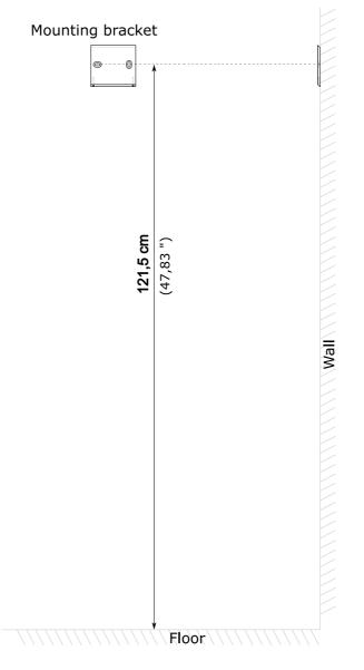
Before installing the TAB10b device:
