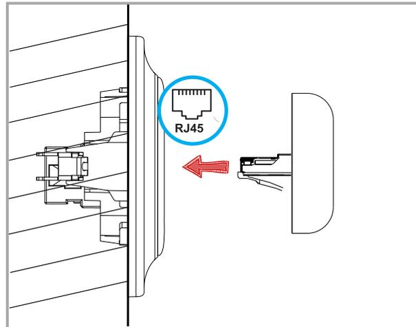
Given the device footprint, it is preconised to use Ethernet wall plug plastron with a right insertion.
