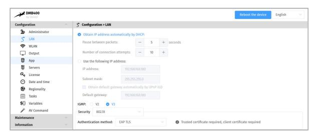
The connection to the device configuration Web user interface with the device IPV6 address, computed from the device MAC address value, is supported. For example, if the LAN MAC address of the device is 00-1c-e6-02-27-bf, type the URL http://[fe80::21c:e6ff:fe02:22ad]/ or type http://[fc00::21c:e6ff:fe02:22ad]/ in a Web browser. The routable prefix is depending on your network configuration.
