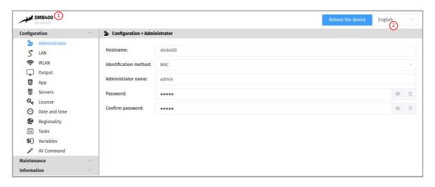
△ After you have changed and saved all your settings in the different panes, be sure to perform a device restart by clicking on the Reboot the device (2) button so that your changes are fully reflected.
