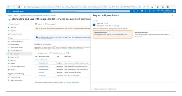
In the display filter input, enter the text  $\it Files$  and check the option  $\it Files.Read.All$ .
