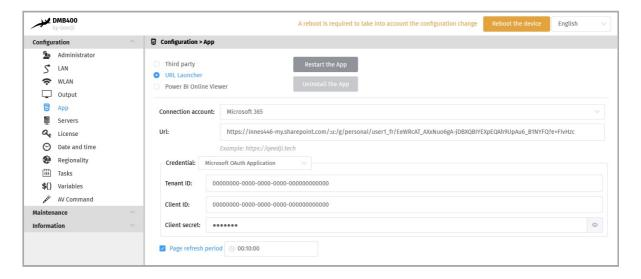
■ In case this information message is displayed on the display device Error - Unable to Launch URL (error HTTP 401), please check the consistency of the Microsoft 365 identifier and password and the consistency of the Azure AD application Tenant ID, client ID and secret ID.
