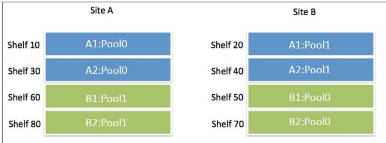
Figure 9) MetroCluster pool-to-shelf assignment.
