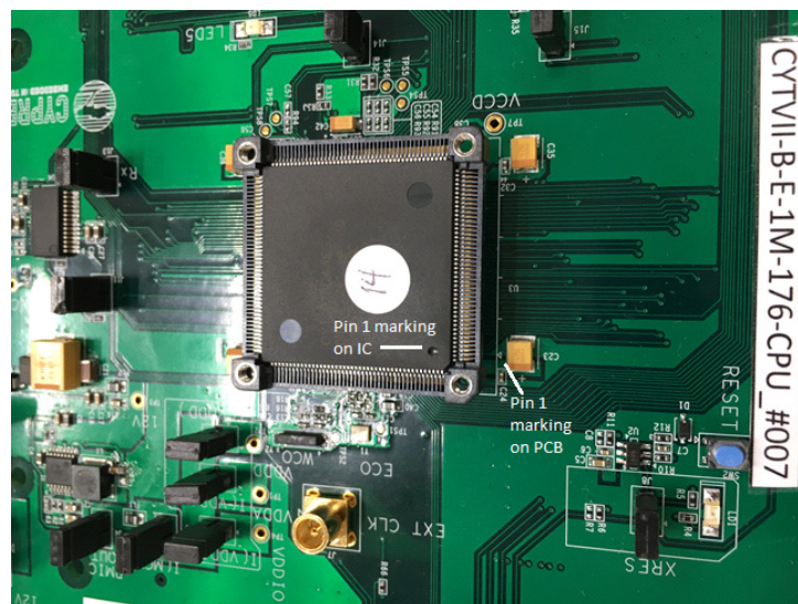
Figure 3-1. Orientation of Device when Inserted in Socket
