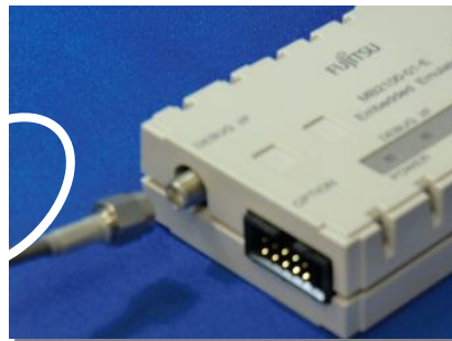
Figure 4-9. Debug Cable Connection to StarterKit
