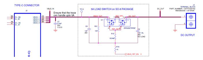
Power supplied by the USB Type-C power adapter is sent to an external device or load through a set of back-to-back Power PMOSFETs. The PMOSFETs are used for the following functions:
