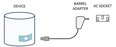
Such electronic devices usually require a specific voltage and current output from the power adapter. To satisfy this, the DC barrel adapter's plug is often custom-made for a device.
