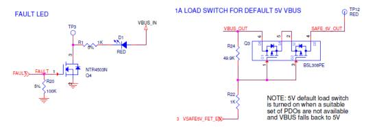
The FAULT LED is turned ON in the following conditions:
