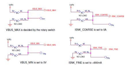
The range of voltages and currents that the BCR device will negotiate with the USB Type-C power adapter is determined by a set of resistor dividers.
