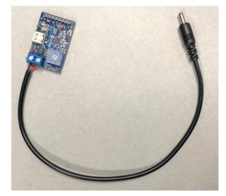
Figure 3-1. CY4533 EVK Connected with Barrel Plug Cable
