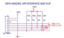
The CY4533 EVK has an 8-pin header (J1) that exposes a few pins, the internal 3.3V rail generated by the BCR device, and ground pins for debug use.
