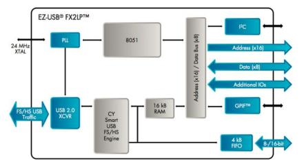
Figure 1. FX2LP Block Diagram
