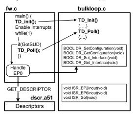
Figure 4. Structure of an FX2LP Application
