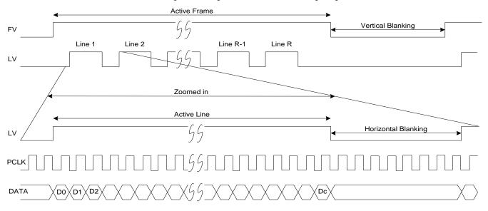
Figure 6. Image Sensor Interface Timing Diagram
