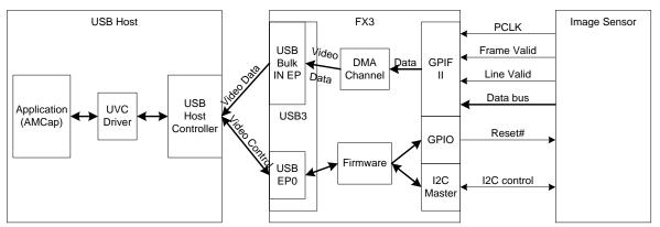
Figure 9. UVC Camera Implementation Using FX3
