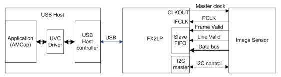
FX2LP provides a master clock (CLKOUT pin) to the image sensor that eliminates the requirement for an extra crystal if the image sensor can use a 12-, 24-, or 48-MHz clock.
