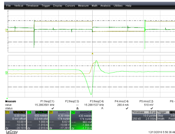
Turn on, V_{ds} and I_{ds} waveform
