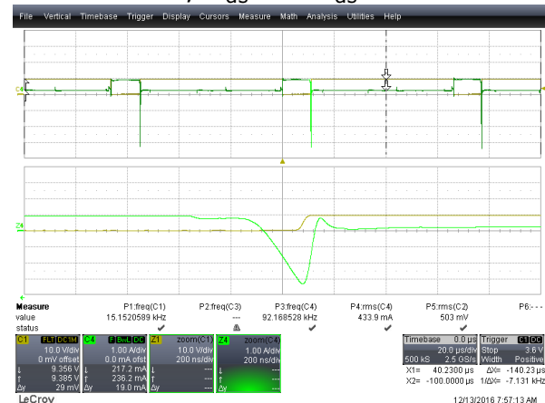
Turn on, V_{ds} and I_{ds} waveform
