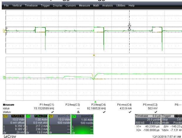
Turn off, V_{ds} and I_{ds} waveform
