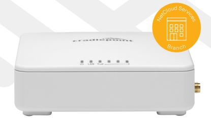
Designed for remote sites that require secure, reliable failover connectivity in the event of a primary link disruption, the CBA550 Series LTE Adapter is a simple addition at the branch which significantly improves uptime and business continuity. These sophisticated devices can be configured at scale with NetCloud to offer a full range of zero-touch deployment, troubleshooting, and management features and integrate into existing configurations.
