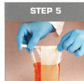
STEP 5 Fold both wire ends onto the bag to provide airtight and leak-proof closure.
