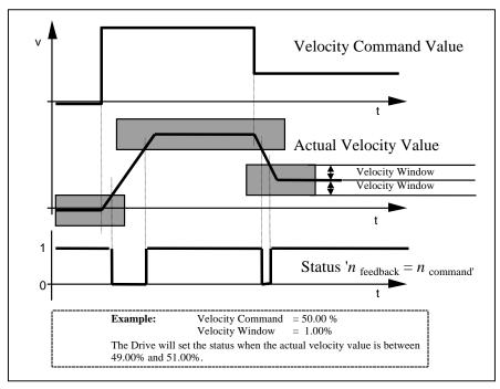
Figure 5.4 - Example of Velocity Window
