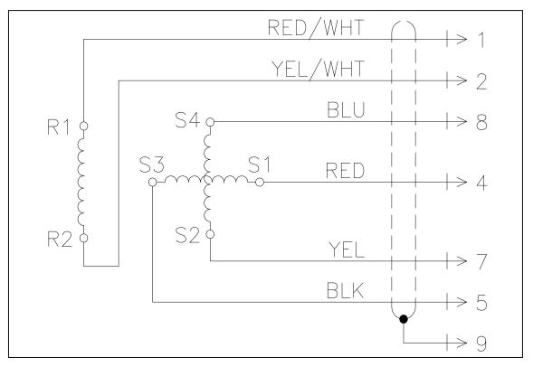
Figure 3.6 - Standard Resolver Wiring Connections for DBM-D100/30R Through DBM-D800/30R
