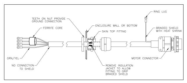
Figure 13.5 - Grounding Motor Armature Cable
