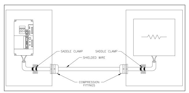
Figure 13.9 - Saddle Clamp Method of Grounding
