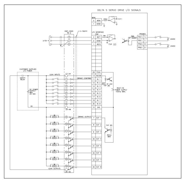
Figure 7.2 - I/O Connections To a DINT-300S
