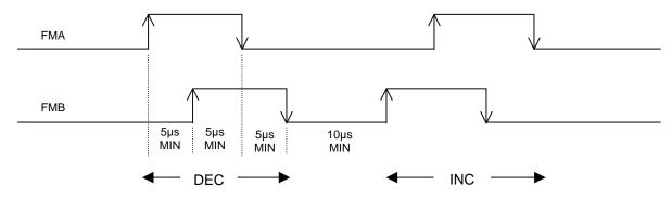
**PULSE AND DIRECTION DECODING (UP-18 = 02)** where FMA is pulse count and FMB is direction. Maximum frequency of FMA is 200 KHZ.
