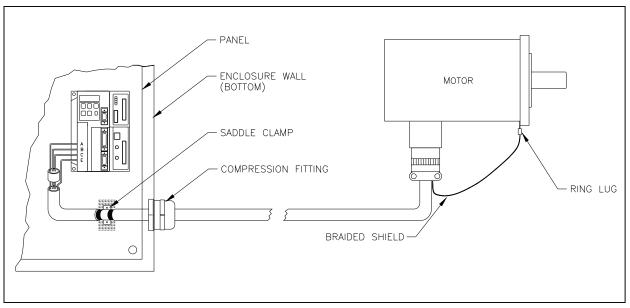
Figure 13.6 - Alternate Method to Ground the Motor Armature Cable
