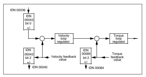
Figure 5.1 - Velocity Polarity Parameter
