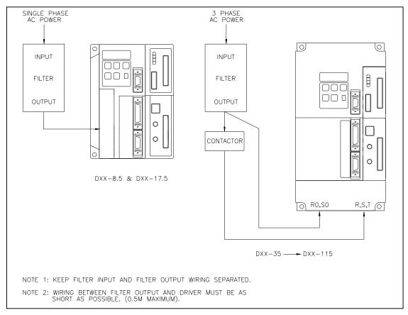
Figure 13.2 - Power Line Filter
