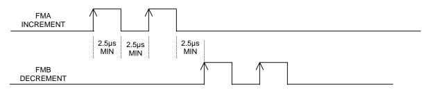
**PULSE-PULSE DECODING (UP-18 = 10)** where FMA decrements the command position and FMB increments the encoder position. Maximum frequency of FMA and FMB is 200 KHZ.
