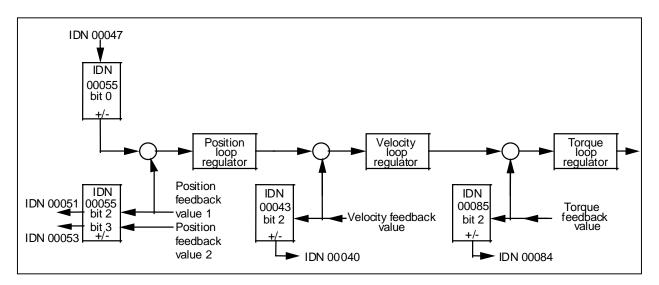
Figure 5.2 - Position Polarity Parameter
