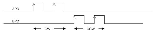
**AB QUADRATURE DECODING (UP-19 = 01)** where APD leads BPD for CCW motor rotation. Maximum frequency of APD and BPD is 100 KHZ. This mode simulates an encoder output being read as 4X.
