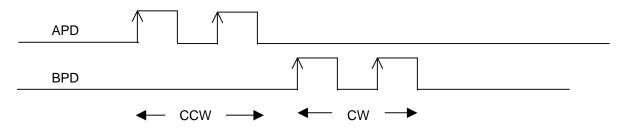
**PULSE-PULSE DECODING (UP-19 = 10)** where APD pulses when the motor actual position moves CW and BDP pulses when the motor actual position moves CCW. Maximum frequency of FMA and FMB is 400 KHZ.
