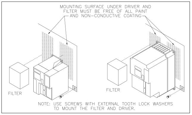
Figure 13.1 - Enclosure Mounting Panel
