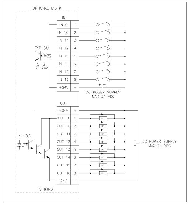
Figure 7.5 - I/O Connections For Optional K (Sinking) Board
