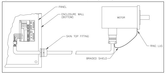
Figure 13.4 - Grounding Motor Armature Cable
