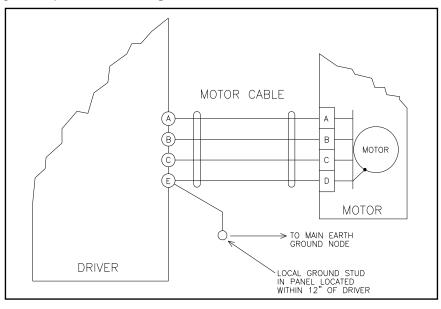
Figure 6.1 - Grounding Technique
