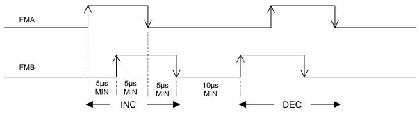
**AB QUADRATURE DECODING (UP-18 = 11)** where FMB leading FMA increments the command position, FMA leading FMB decrements the encoder position. Maximum frequency of FMA and FMB is 50 KHZ.
