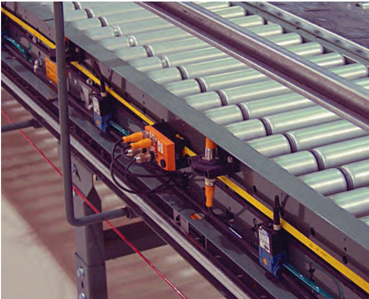
The AS-i network connects hundreds of sensors on a single two-wire cable. AS-i I/O modules use quick plug-and-play functionality that simplifies installation.
