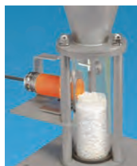
The KI and KG sensors detect granulars such as plastic regrind.
