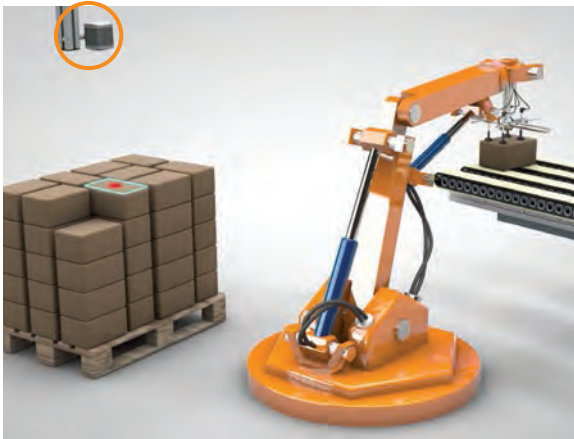
The next box is located during the previous cycle, to eliminate dwell time.
