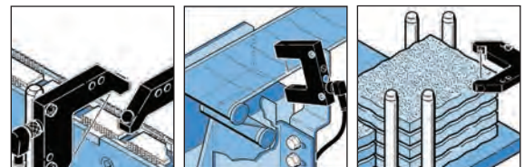
Detection of legs on integrated circuits
