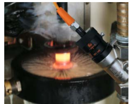
Mechatronic sensor in the coolant circuit of an induction furnace.
