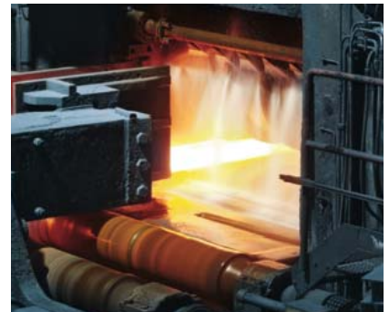
Position detection of steel slabs in a rolling mill.
