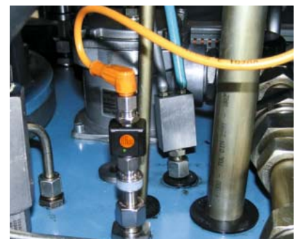
Use of a modular TP transmitter instead of a common head / DIN rail transmitter.
