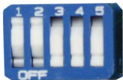
Figure 2-3: DIP switch set to Decimal Address 3
