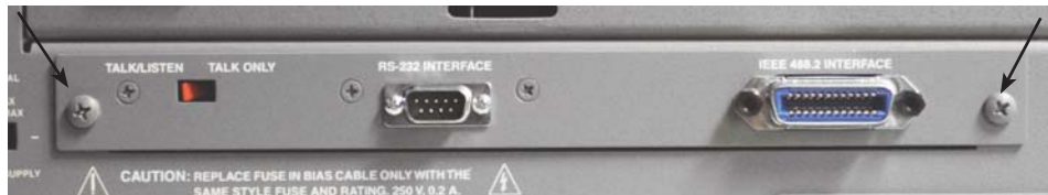
Figure 5-9: Screws holding the interface assembly on the rear panel
