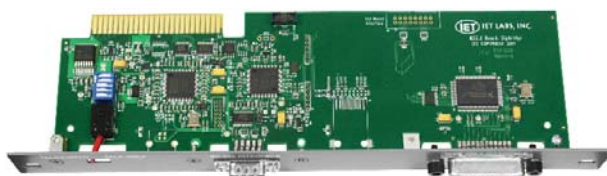
Figure 5-8: IEEE interface (1689-9640), top view
