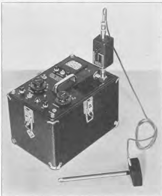
The vibration pickup and control box plug into the sound-level meter in place of the microphone, as shown here.
