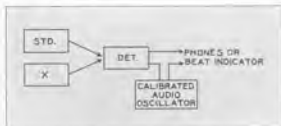
FIGURE 6. Functional diagram showing the operation of the direct-beating method of frequency measurement.
