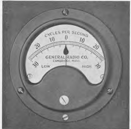
View of the deviation indicator, showing the open, easy-to-read scale.
