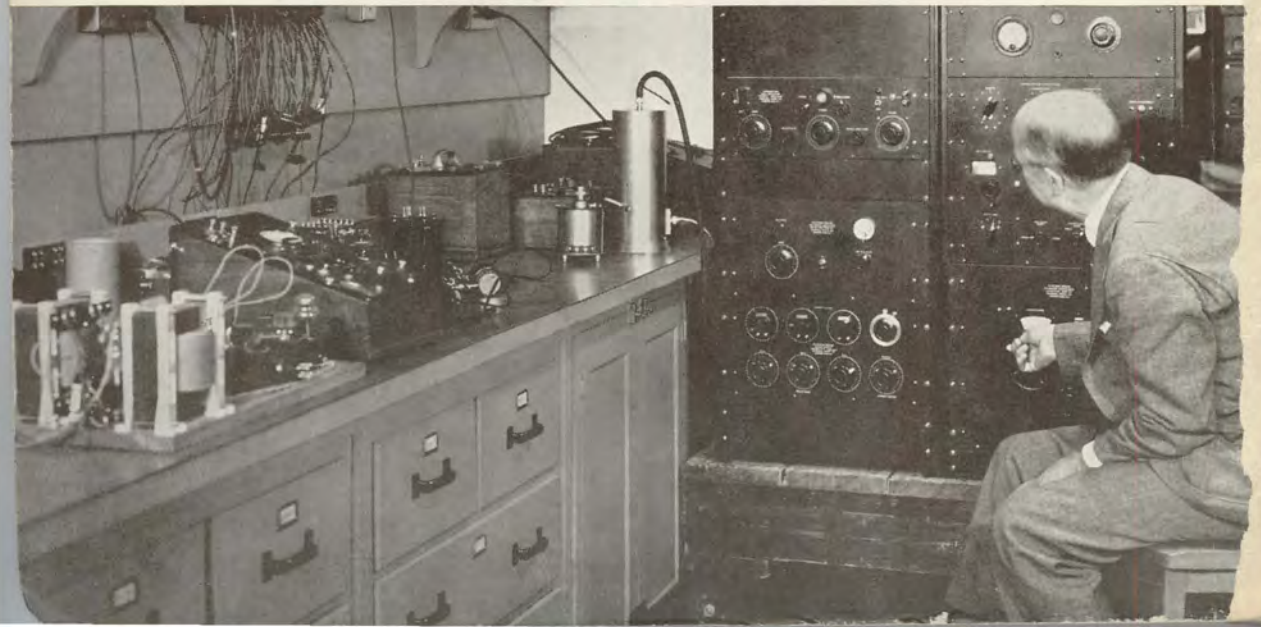
Above—Measuring frequencies with the General Radio Primary Standard of Frequency. Below—Engineering tests on a high-voltage, 60-cycle Schering Bridge.
