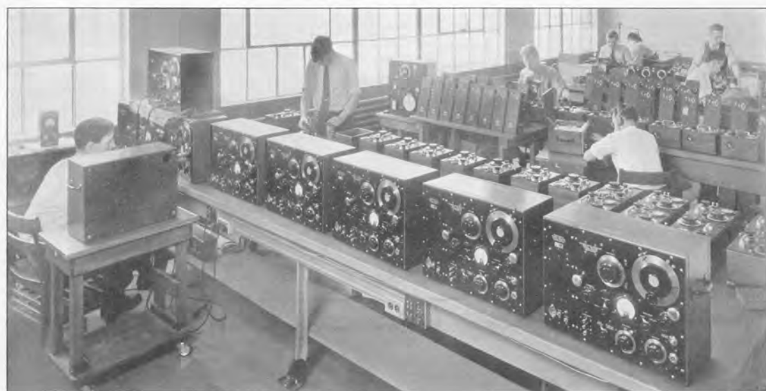
Calibrating and testing TYPE 605-B Standard-Signal Generators in the General Radio Standardizing Laboratory.
