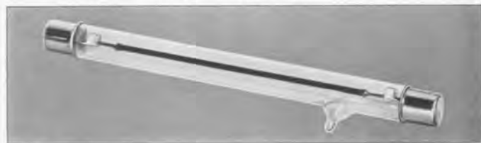
View of the high resistance standard used in TYPE 729-A Megohmmeter.
