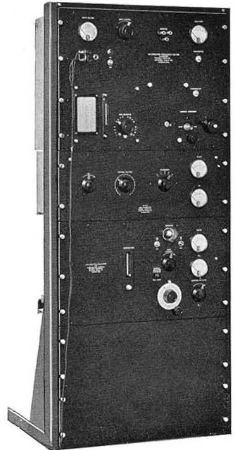
A Class C-10 Standard-Frequency Assembly with a TYPE 616-AR Heterodyne Frequency Meter (upper panel) makes a frequency-measuring equipment that is complete, except for the necessary radio receiver
