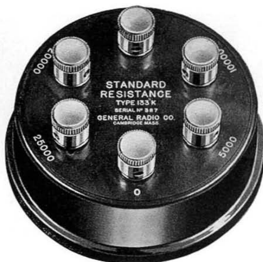
A TYPE 133-K Standard Resistance having a resistance of 25,000 ohms tapped at the four, 5000-ohm points
