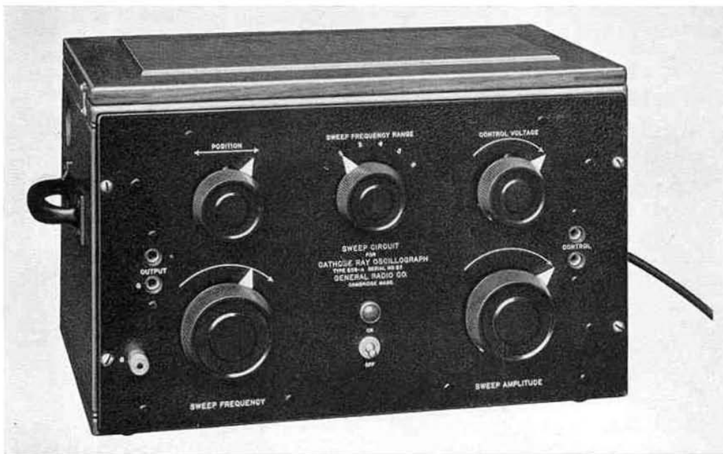
This sweep circuit supplies a linear time axis for the cathode-ray oscillograph. Linearity, wide frequency range, and a-c operation are its principal features
