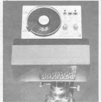
The control unit and lamp-head assembly can be attached together and mounted on a tripod for convenience or, with the neck strap supplied, can be made as portable as you need dictates.
