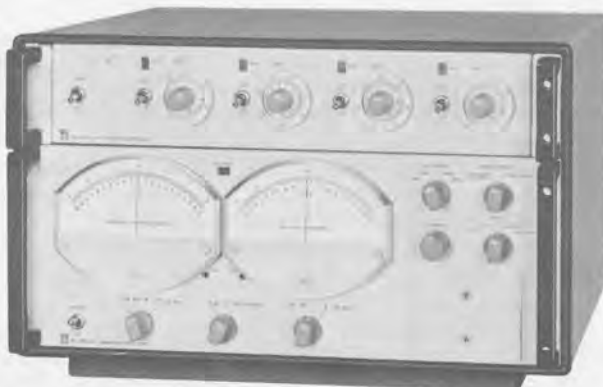
The 1782 is shown here with the 1654 Impedance Comparator to form one version of the 1654-Z Sorting System.
