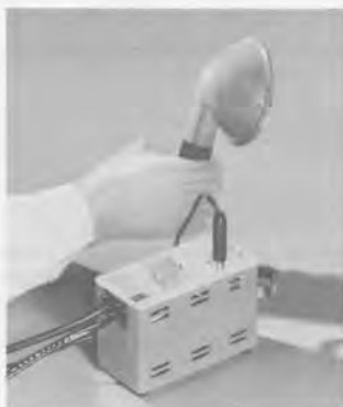
The lamp can be removed from its clamp at end of case and hand-held up to 5 feet away.
