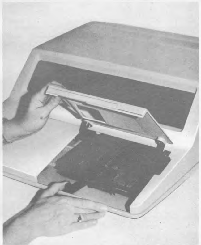
Installing a program board.
