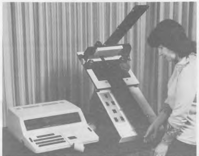
GR 1742 interfaces to a variety of automatic handlers.
