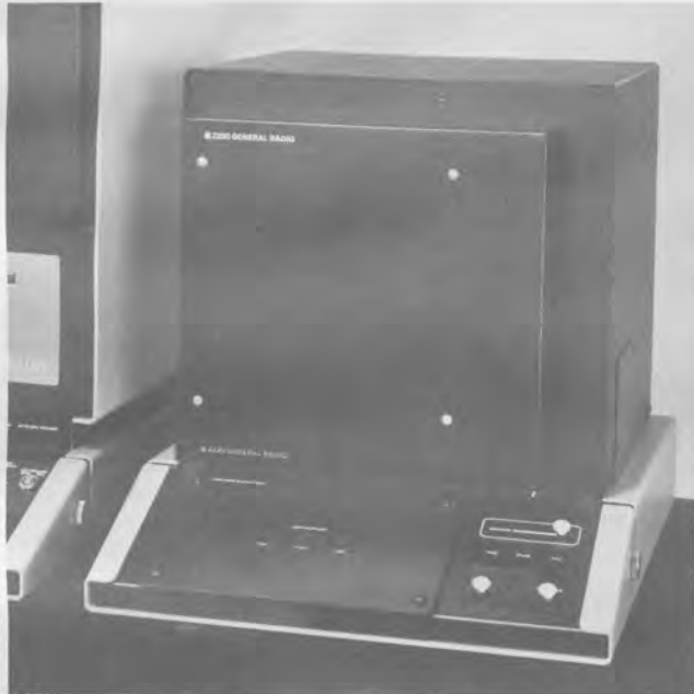
For increased scanner capability beyond 32 channels, this test console is used to house additional scanner boards.
