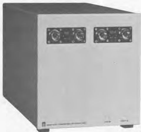
1408 standard, with temperature-controlled air bath.
