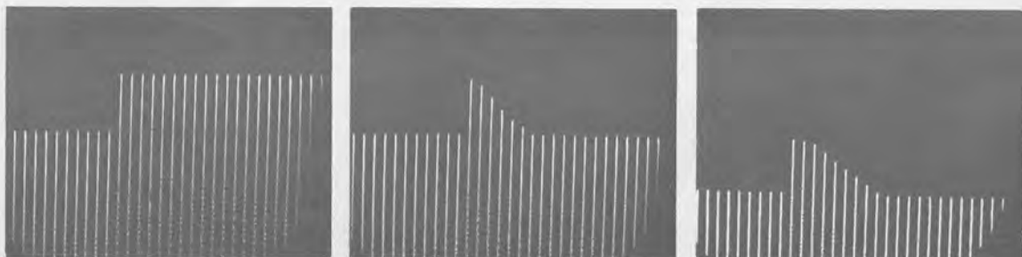
Oscillograms of line-voltage peaks show response speed of Variac® automatic voltage regulators: left, 2% step change in line voltage; center and right, resulting output transients for 1581 and 1582 Regulators, respectively.
