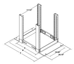
Equipment rack options self-support bases are 3-1/2" x 6" extruded aluminum angles mounted at the bottom of all standard equipment racks.
