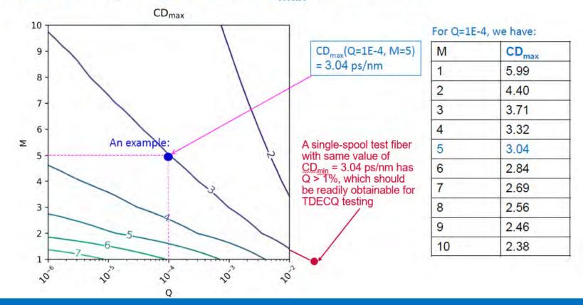
Because of the significant relaxation of  $CD_Q(M=5, Q=1e-4)$  relative to the worst case, a 10 km single-spool test fiber (M=1) with the same value of CD has Q > 1%. This means that such a test fiber should be readily obtainable, since it represents >1% of fiber vendors' production. This is a vast improvement over trying to obtain a 10km test fiber with 9.2 ps/nm CD, or having to use up to >30 km of nominal fiber in the test set.
