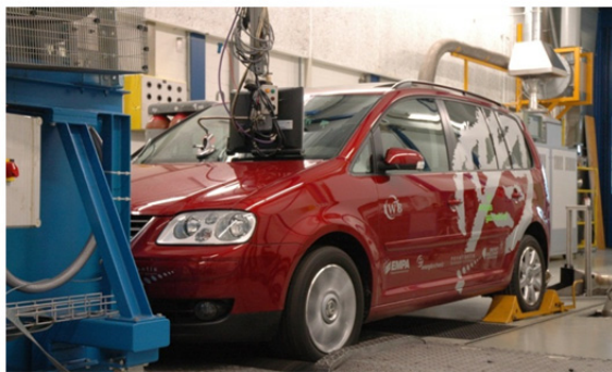
Fig. 5 Euro 4 Passenger Car with 2.0-L Engine and Conventional Three-Way-Catalyst Being Tested with 15% and 25% Vol H 2 in CNG
