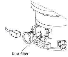
Air inlet valve P/N 24 V DC 114280
