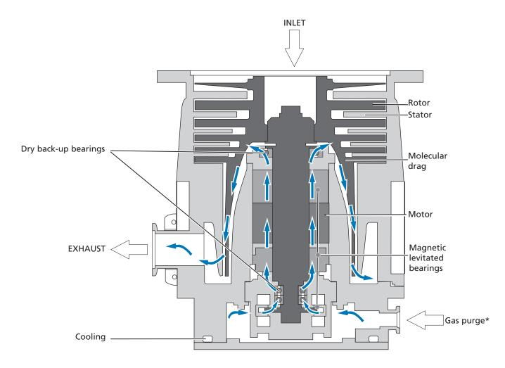
\* The gas purge provides an excellent protection of the maglev bearings for corrosive applications and ensures the rotor cooling.
