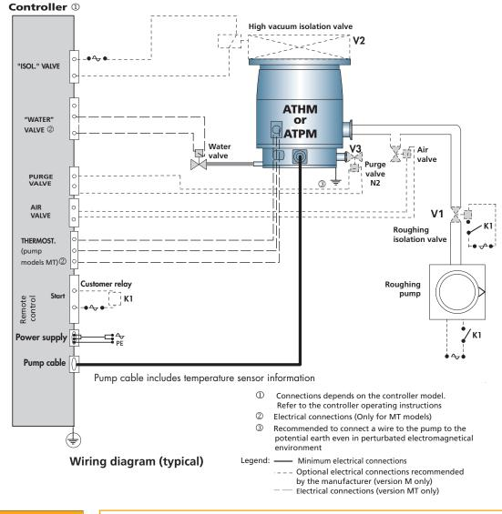
We recommend that you fit a separate earth (ground) conductor to earth pump. Use an un-insulated braid or a separate insulated green/yellow conductor with a minimum 9AWG (3mm2) conductor (to comply with US and Canadian installation codes). Use a screw and a shakeproof washer fitted to the earth hole from the pump to secure the earth conductor to the pump. The impedance between the pump-body and the earth connection point must be < 0.1 Ohm at 25A.
