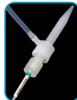
Sample capillary attached to PFA Nebulizer
