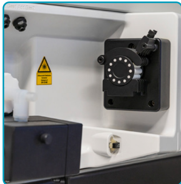
MP 2 peristaltic pump installed on an iCAP™ Q ICPMS
