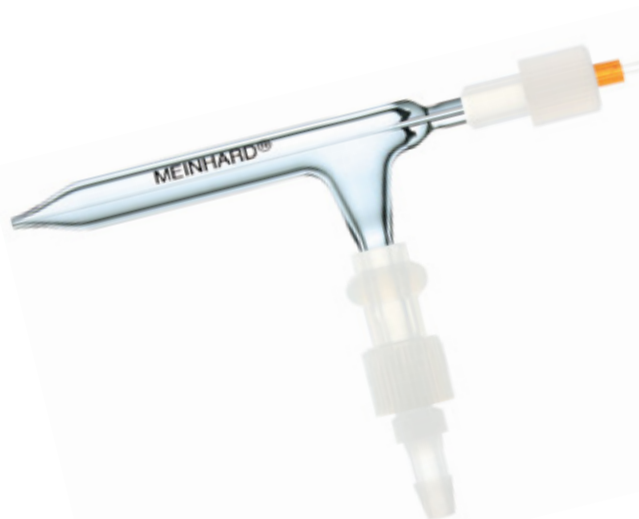
MEINHARD® SilQ+ high purity nebulizer with FG+ PFA gas fitting TQP-50-A0.5
