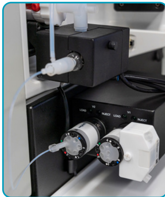
Integrated capillary nebulizer and prepFAST with SampleSense on an iCAP™ RQ
