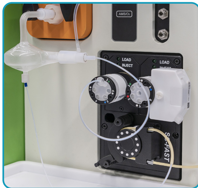
Integrated capillary nebulizer and prepFAST with SampleSense on a NexION 2000 ICPMS
