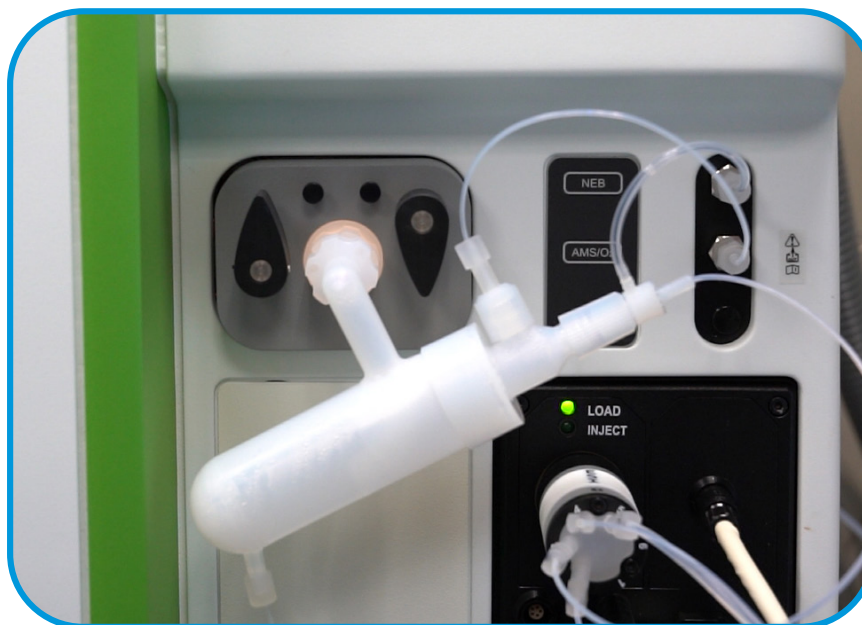
Fluorospray Sample Introduction Kit assembled on NexION 5000 ICPMS
