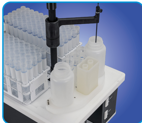
Extra position can be used for static rinse, organic rinse, or additional sample or tuning locations
