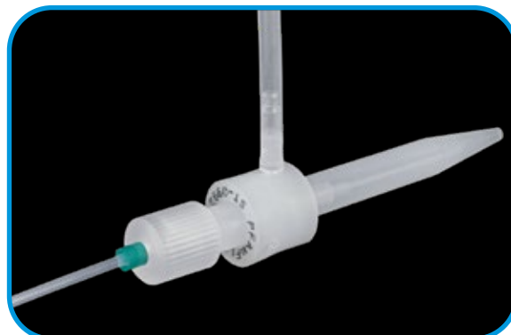
Sample capillary attached to PFA-ST MicroFlow nebulizer
