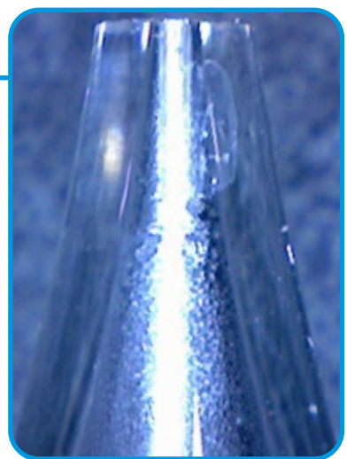
Water microdroplets continuously clean the inside of the nebulizer and prevent salt deposits.
