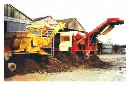
Figure 5 Sugar beet cleaner/loaders with manned pick-off platforms
