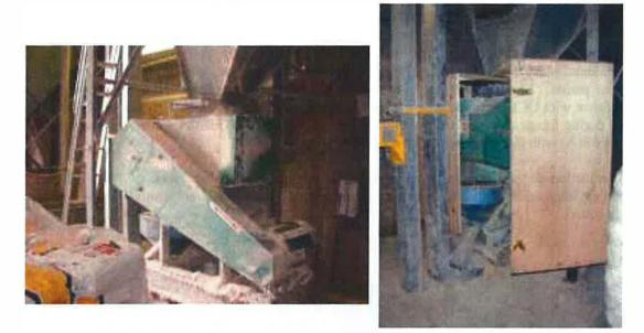
Figure 17 Animal feed cubing machine installation, before (left) and after (right) noise reduction treatment (noise reduction enclosure shown open for machine maintenance)
