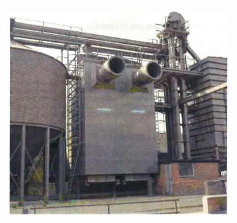
Figure 7 Large, continuous-flow grain drying installation
