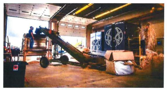
Sample decorticated equipment been fed hemp stalk and outputting processed material.
