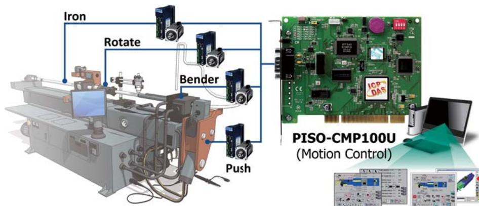
In the machine, there are six-axis motors which use distributed CANopen motion control. During the tube bending process, the two axes of the feeding and radial bending are designed to be interpolation motion. The cycled processes are designed to prevent the metal tube broken and rebound. It greatly improves the yield of bending. The CANopen motion also help to shorten the development time at the design stage.
