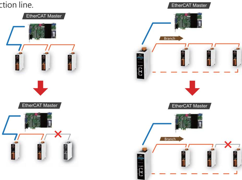
▲ If there is no diverter, the module will stop working when the cable disconnects.
