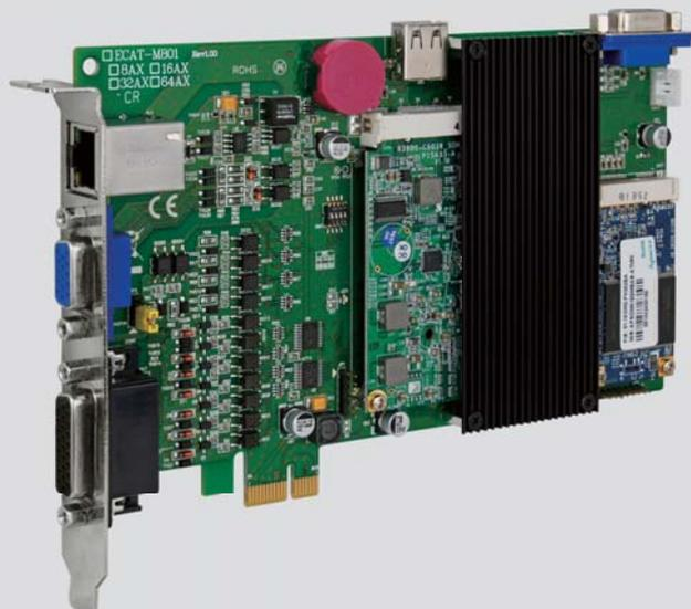
▲ ECAT-M801 handles motion control, allowing the PC system to focus on other tasks
