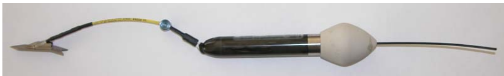
Fig. 3.3.1.1. Mk10-PAT tag equipped with a metallic dart (photo by M. Deflorio)
