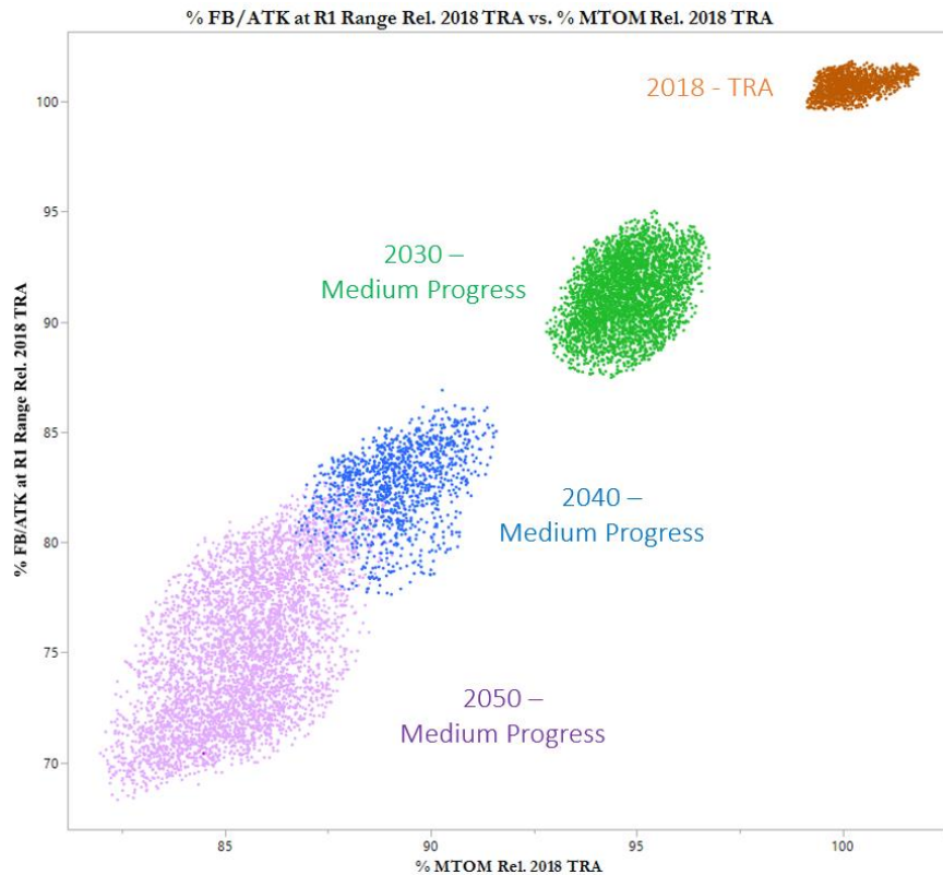
Figure 5-6. WB ATW Optimization Clouds for Medium Progress
