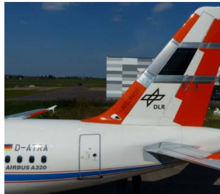
Figure 4-3. AFLoNext HLFC empennage flight test on DLR's A320 test aircraft
