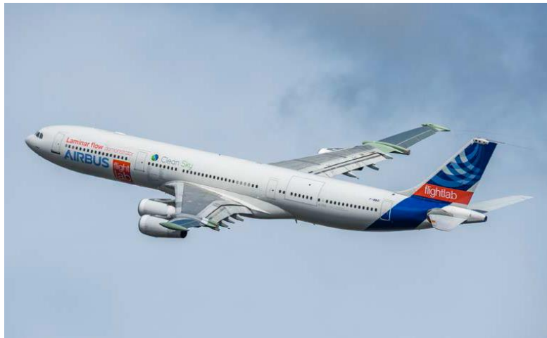
Figure 4-2. Integrated wing NLF (Natural Laminar Flow) integration concepts installed on modified outboard wings of Airbus A340-300 (Clean-Sky 2 flight demonstrator BLADE)
