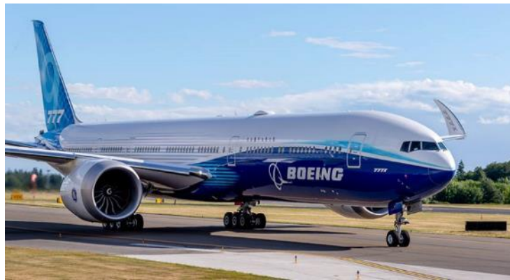
Figure 4-1. On-ground folding wing tip to maximize in-flight wing span (Boeing B777-9)
