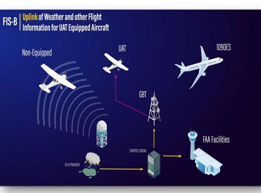
The yellow arrows show ground-based data flow from the Flight Planning systems to the control station, then the ground-based towers (GBT). The pink arrows show the transmitted data flow to UAT equipped aircraft.
