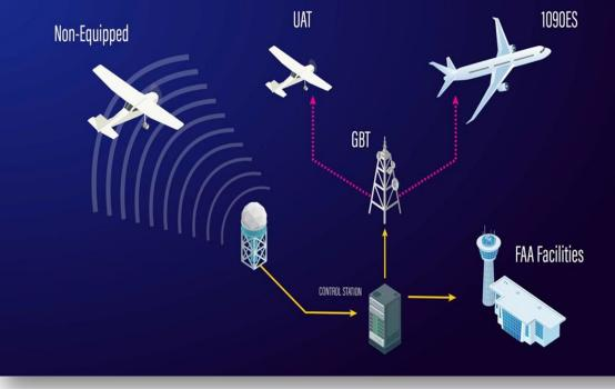
The yellow arrows show ground-based data flow from the receiver about non-ADS-B equipped aircraft to the control station, then the ground-based towers (GBT). The pink arrows show the transmitted data flow to ADS-B equipped aircraft.
