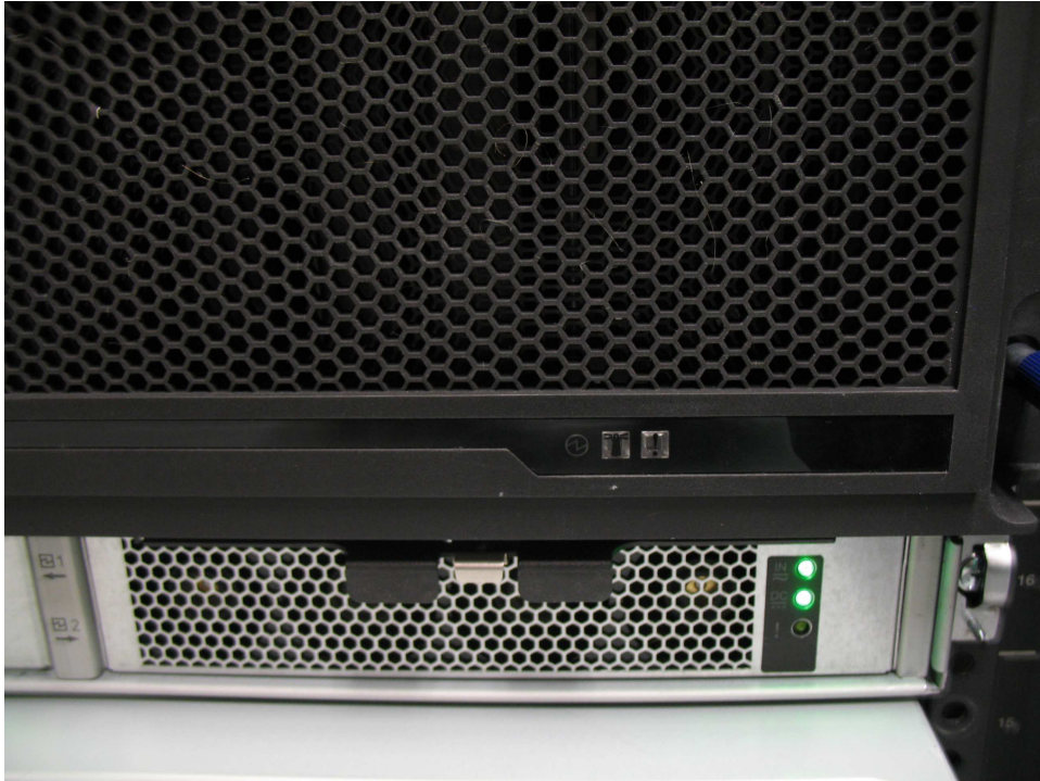
Figure 71. Fascia removed from the PSUs
