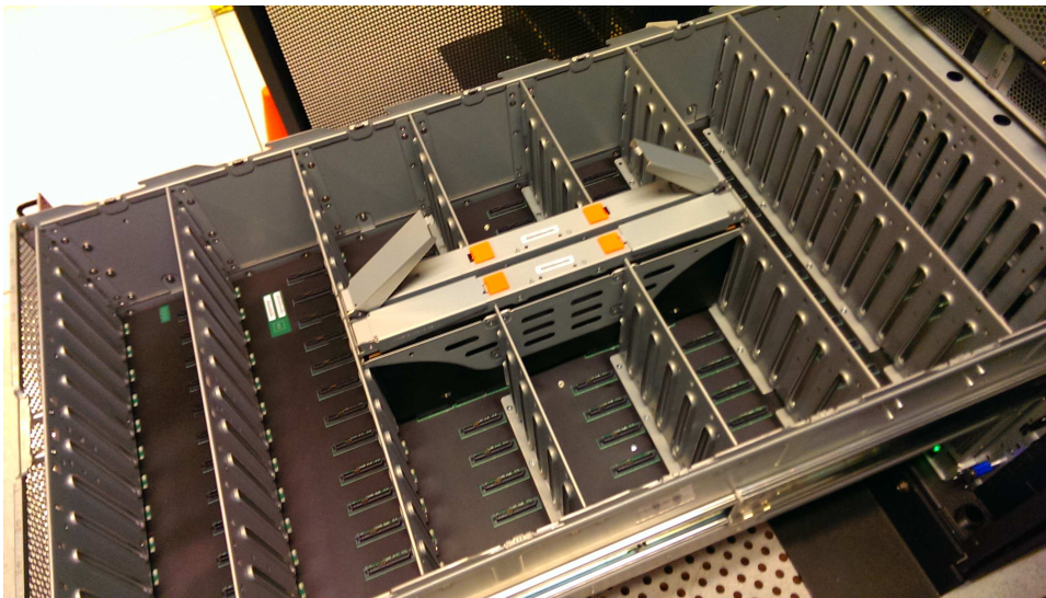
Figure 112. Location of secondary expander modules
