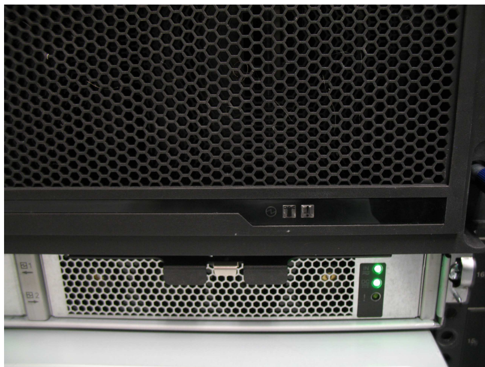
Figure 120. Power supply indicators
