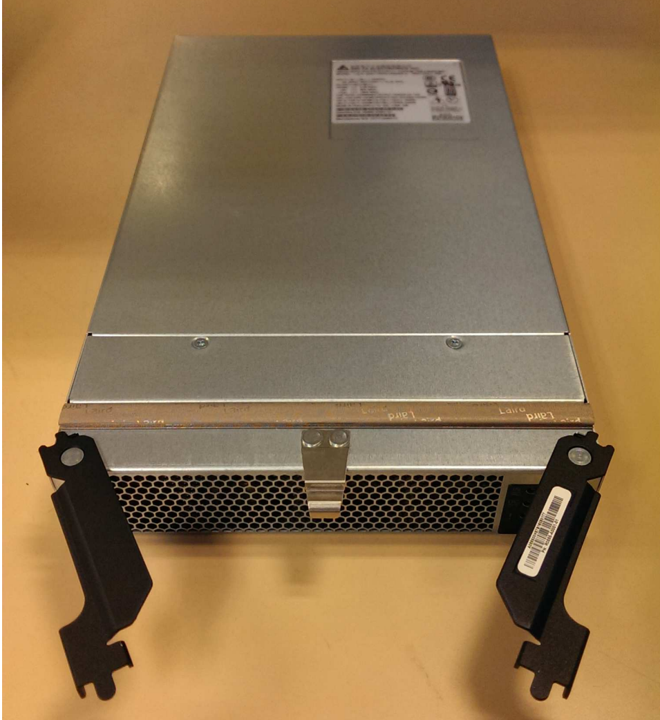
Figure 73. Removed power supply
