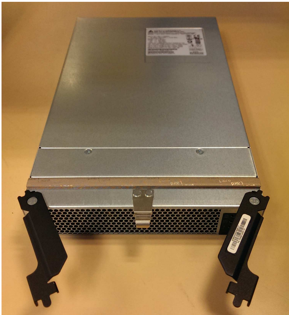
Figure 118. Preparing to install the power supply
