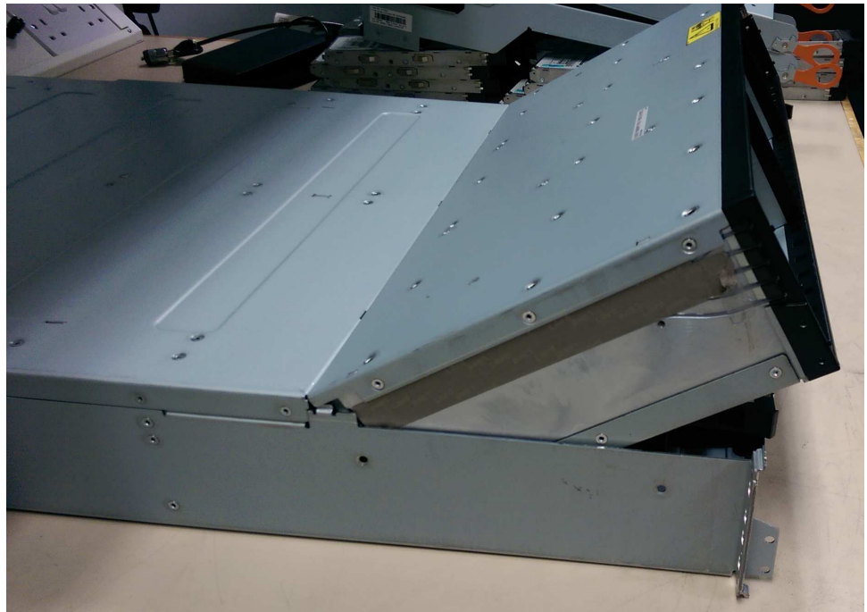
Figure 36. Angled midplane assembly
