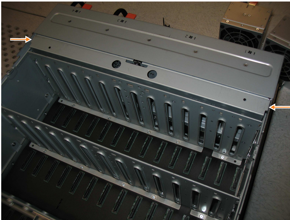
Figure 85. Location of the FIB cover
