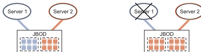
Figure 4. Minimal configuration of two IBM Spectrum Scale RAID servers and one storage JBOD. IBM Spectrum Scale RAID server 1 is the primary controller for the first recovery group and backup for the second recovery group. IBM Spectrum Scale RAID server 2 is the primary controller for the second recovery group and backup for the first recovery group. As shown, when server 1 fails, control of the first recovery group is taken over by its backup server 2. During the failure of server 1, the load on backup server 2 increases by 100% from one to two recovery groups.
