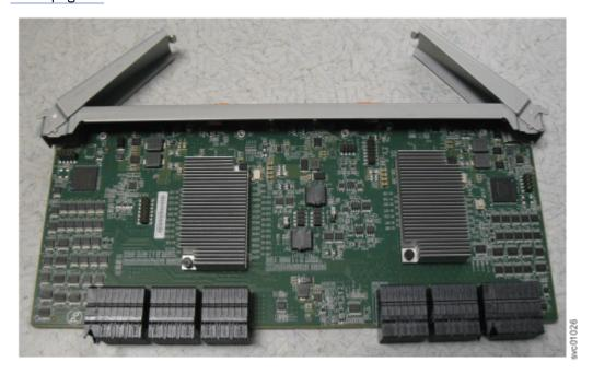
Figure 88. Open the secondary expander module handles
