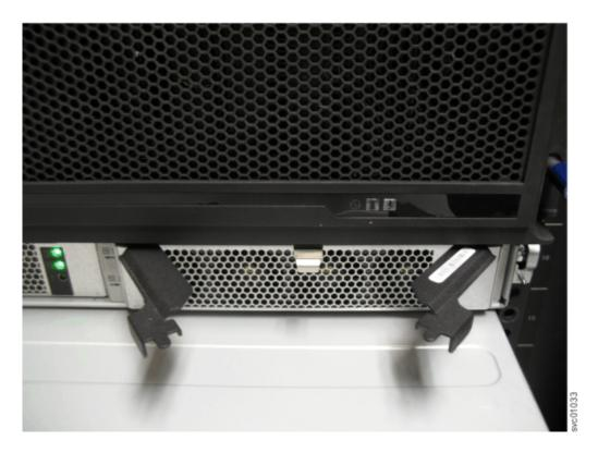
Figure 108. Releasing the power supply handles
