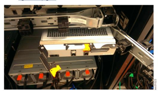
Figure 63. Install the expansion canister
