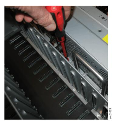
Figure 105. Secure the FIB to the drive board
