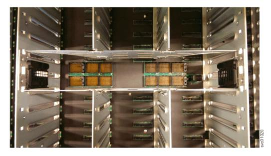
Figure 116. Secondary expander module connectors
