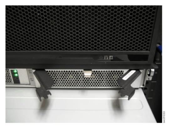
Figure 93. Install the power supply
