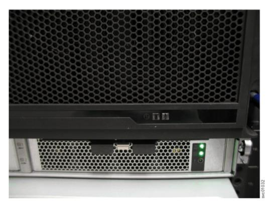
Figure 97. Fascia removed from the PSUs
