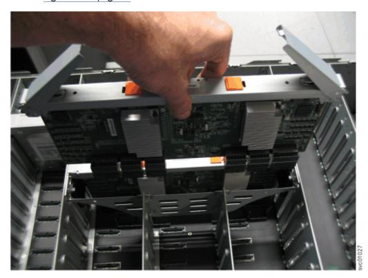
Figure 89. Replace the secondary expander module
