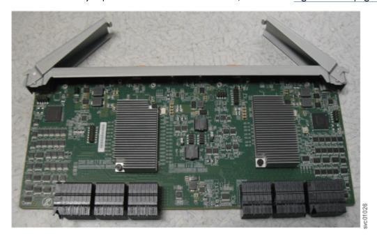
Figure 117. Secondary expander module removed from the enclosure
