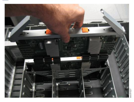
Figure 115. Remove the secondary expander module
