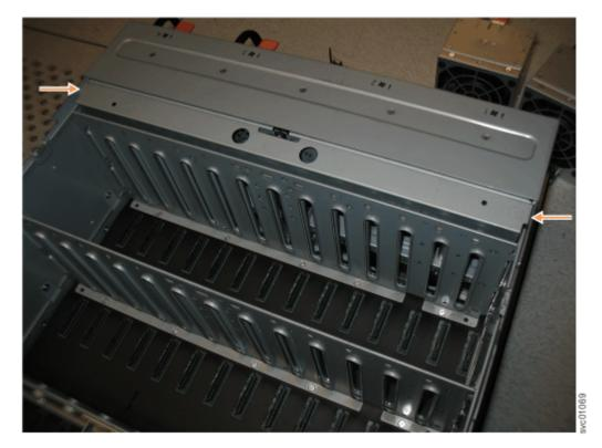
Figure 106. Replace the FIB cover
