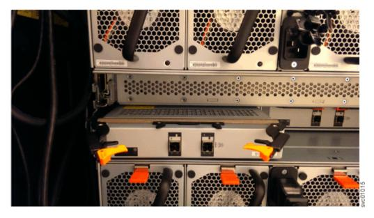
Figure 119. Removing the expansion canister
