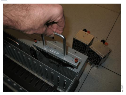
Figure 126. Remove the FIB from the chassis
