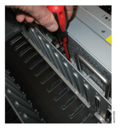
Figure 125. Loosen the FIB screws
