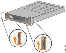
2. Align the enclosure with the front of the rack cabinet.
