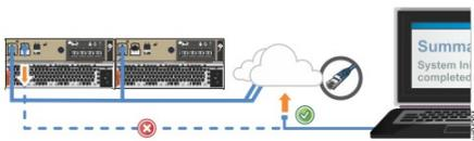
Ethernet port 1 remains connected to the network, as shown. Ethernet port 2 no longer acts as the technician port.
