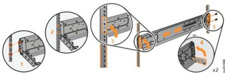
9. On the front of the rail, press the two bracket pins into the holes in the rack flanges.
