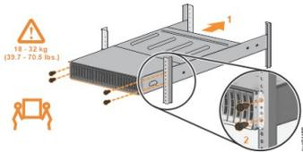
**Note:** The rails are not designed to hold an enclosure that is partially inserted. Always fully insert the enclosure in the rack.
