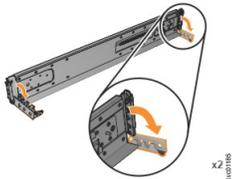
6. Align the holes in the rail bracket with the holes on the front and rear rack cabinet flanges. Ensure that the rails are aligned on the inside of the rack cabinet.
