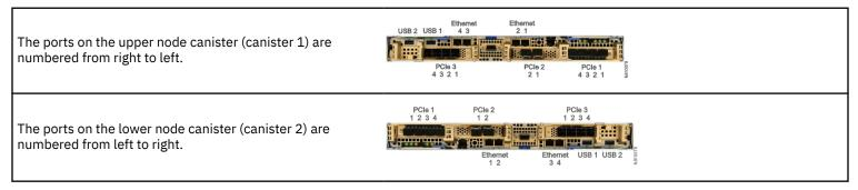
Use the following table to record the properties of the onboard Ethernet ports on each node canister of the control enclosure. The configuration of the onboard Ethernet ports for FlashSystem 7200 and Storwize V7000 Gen3 systems are the same.
