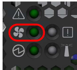
Figure 56: Fan Status LED in SN2700 - Front and Rear Sides
