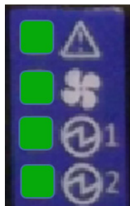
Figure 48: System Status LEDs 5 Minutes After Power On in SN 2100
