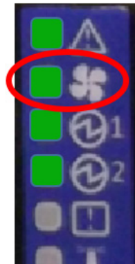
Figure 58: Fan Status LED in SN2100
