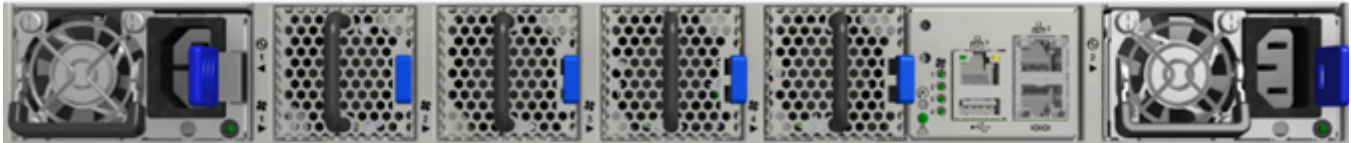
Figure 6: Air Flow Direction Marking - Power Side Inlet to Connector Side Outlet
