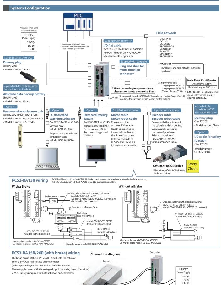
The cable is to be prepared by the user. The connector is included \* For details, please refer to the instruction manual.
