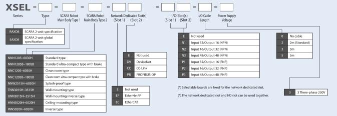
Note: When the brake option is selected with IX-NNN or NNC 1205/1505/1805, be sure to specify the model number of the IX type with the brake option (1205B/1505B/1805B).
