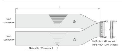
\* Enter the cable length (L) into  $\Box\Box\Box$  . Compatible to a maximum of 10m. Ex.: 080=8m
