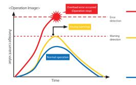
The increase and excessive load of the sliding resistance due to the lack of maintenance of the guide and the ball screw increases the current applied to the motor. **As a result, an overload error occurs and the device stops.**
