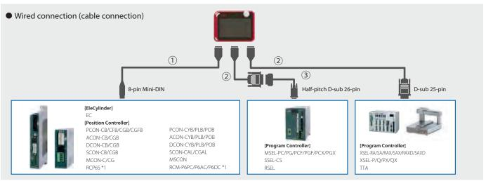
\*1 To operate RCP6S and RCM-P6, a gateway unit or a PLC connecting unit is necessary.
