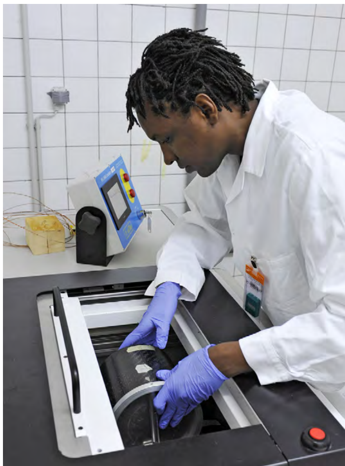
Agency research scientist using an X-ray machine to irradiate larger organisms at lower doses.
