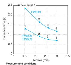
Distance from measurement point: 300 mm Ionization time: ±1,000 V to ±100 V Plate monitor: 150 × 150 mm, 20 pF
