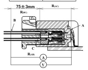
Fig 5.In-line Circuit Test Lead Location
