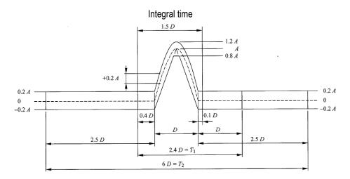
Fig11. Sinusoidal half-wave
