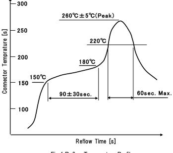
Fig.1.Reflow Temperature Profile
