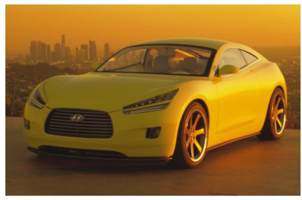
The HCD8 with its supercharged 2.7-liter V6 engine, 6-speed manual transaxle and tuned dual exhaust provides performance to match its styling. For real world driving, the driver can adjust the ride height a total of four inches through the air suspension. The vehicle can sit low for high-speed touring or can be raised to handle inclement weather, avoid barking wheel stops, handle a car wash or any other situation where additional ground clearance is needed.
