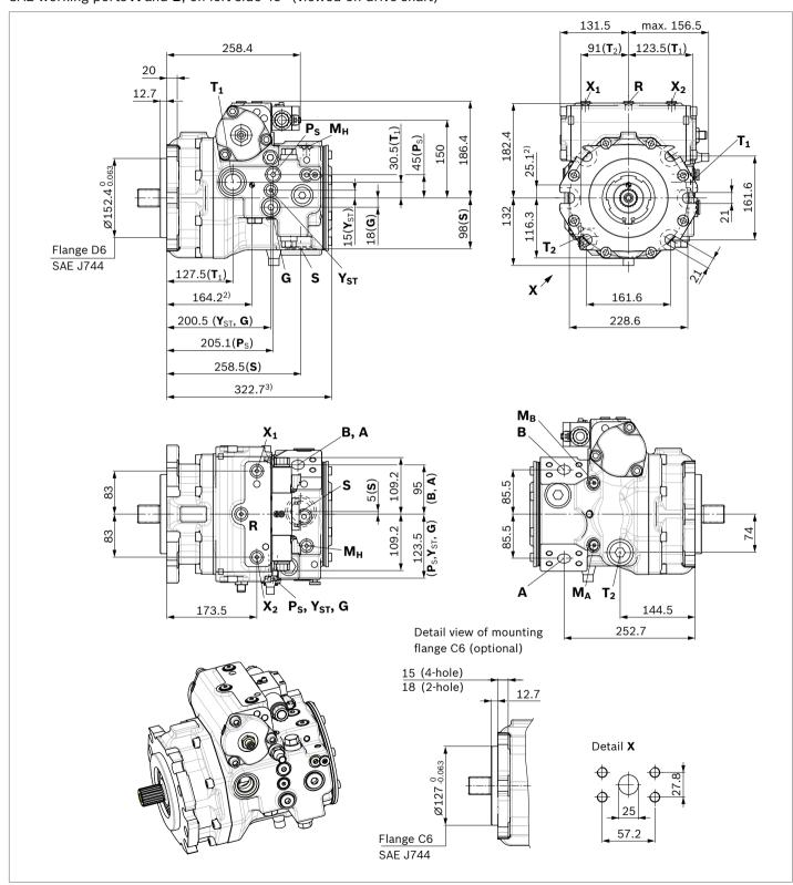
$_{\rm 1)}$  For SAE working ports  ${\bf A}$  and  ${\bf B},\,45^{\rm o}$  right (viewed on drive shaft), the complete case and thus the dimensions are mirrored.
