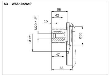
Involute spline according to ANSI B92.1a, 30° pressure angle, flat root, side fit, tolerance class 5
