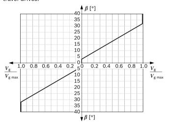
Swivel angle  ${\pmb \beta}$  at the control lever for pump displacement change:
