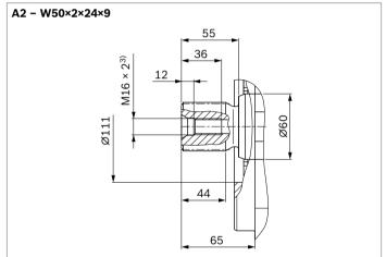
$_{\rm 1)}$  Involute spline according to ANSI B92.1a, 30° pressure angle, flat root, side fit, tolerance class 5
