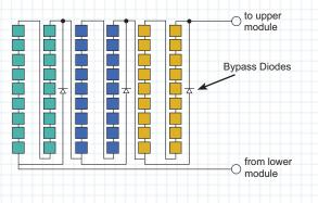
The LX2400 IDEAL<sup>™</sup> Solar Bypass Device with Microsemi's patented CoolRUN<sup>™</sup> technology provides a bypass path in PV module applications with the industry's lowest forward voltage drop resulting in negligible heat generation and temperature rise during operation for best in class reliability and robustness. A scalable architecture provides future-proofing for next generation PV modules operating at higher than 10A currents.
