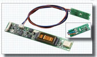
The LXMG181x Series is designed to enhance the current offering: the customer will benefit from a wider input voltage range (VIN) at fully regulated lamp current, and an enhanced Lamp Driving capability (see the range of VLAMP and the Striking capability). Fewer part numbers (4 instead of 24) will be able to drive an extended list of displays thus greatly simplifying the customer supply
