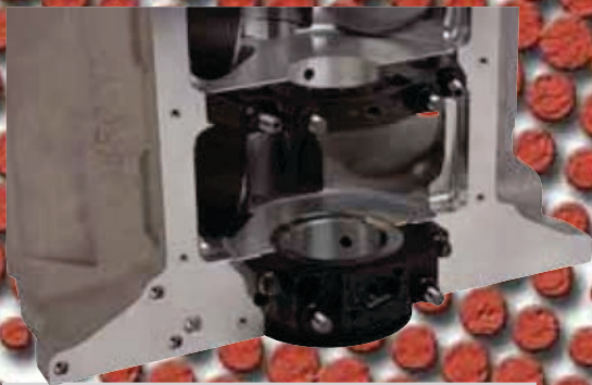
BILLET MAIN CAPS INSTALLED WITH SPLAYED BOLT PATTERN
